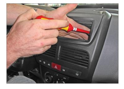
2. Remove 2 screws (left and right)
